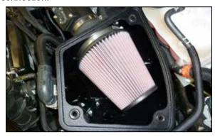
32. Install the K&N air filter onto the filter adapter and secure with the provided hose clamp.
