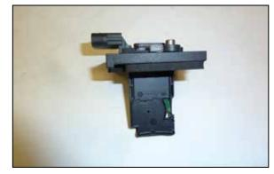
23. Remove the mass air sensor from the factory housing and then install the sensor into the adapter provided along with the gasket.
