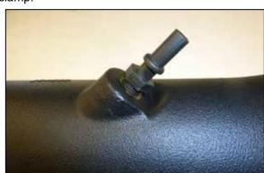
22. Install the provided quick connect fitting into the K&N intake tube.
