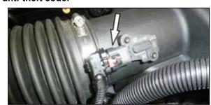
2. Disconnect the mass air sensor electrical connection and loosen the hose clamp that secures the factory intake tube to the air filter housing.
