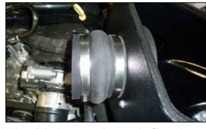
20. Install the hump coupler onto the filter adapter and secure with the provided hose clamp.
