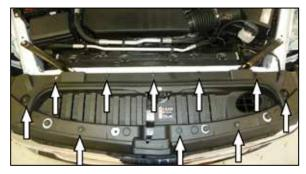
9. Remove the ten push pins that secure the upper radiator valence and then remove the valence from the vehicle.
