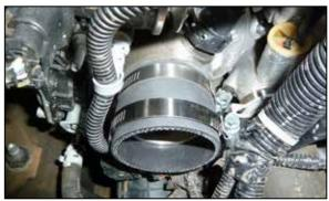
21. Install the provided straight coupler onto the turbo inlet and secure with the provided hose clamp.
