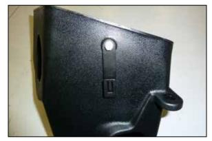
13. Install the provided bulk connector bracket onto the K&N air filter housing and secure with the provided hardware.
