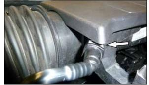
Depress the locking tab and then disconnect the CCV pipe from the plenum.
