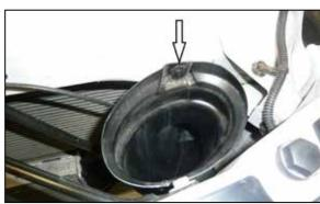
10. Remove the push pin that secures the fresh air duct to the core support and then dislodge the duct from the air filter housing. This push pin will be reused in a later step.
