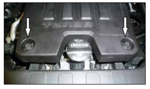
6. Remove the two bolts that secure the engine cover to the engine and then remove the cover from the vehicle. These bolts will be reused in a later step.
