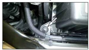
12. Remove the nut that secures the air filter housing to the mounting bracket. This nut will be reused in a later step.
